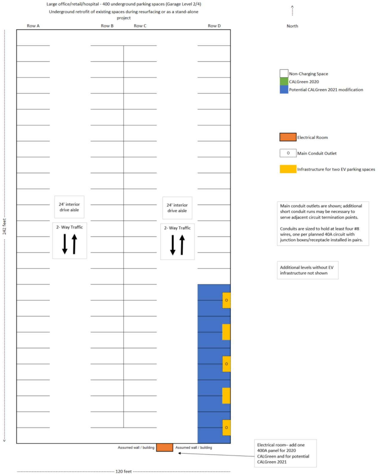
Figure 9. Retrofit scenario of large office/retail/hospital with 400 parking spaces (Level 2/4)
