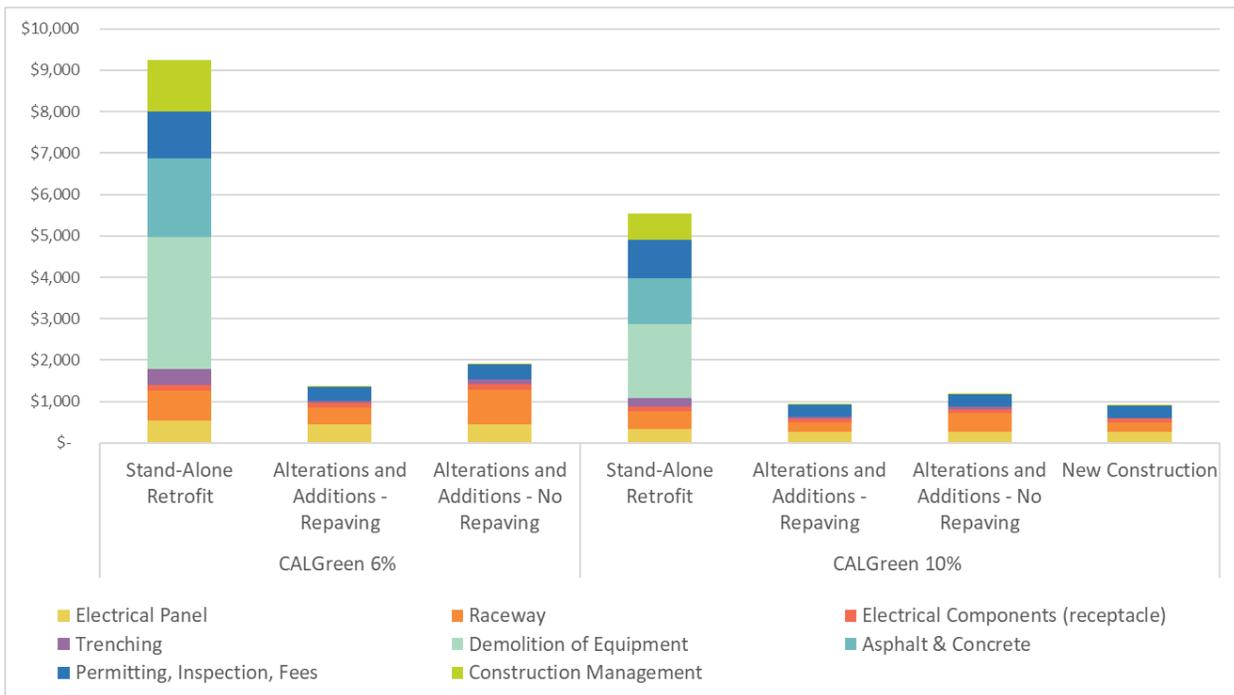
**Figure 2. Cost Break-Down per EV Capable Parking Space - Medium Office/ School**
